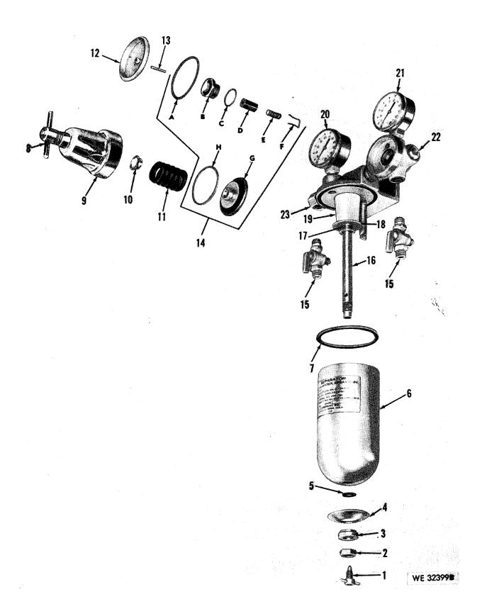
Figure 1. Separator - exploded view
